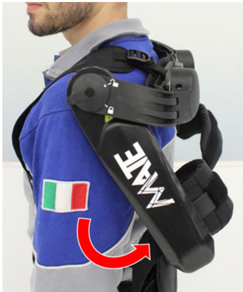
Fig. 3.5 - Torque Generator Box in rear home position. This is the only position where the locking mechanism can be activated or deactivated
