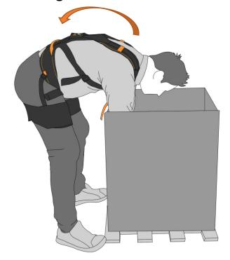
The equipment provides relief of 18 to 28 kilograms, depending on the selected configuration
