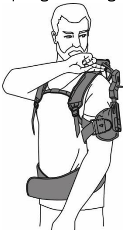
Correct position of spring, two fingers between spring and shoulder
