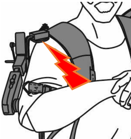
Spring touching the shoulder when arm is moved upward
