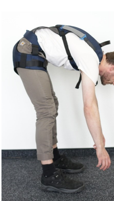
You will feel the assisting force of the LiftSuit on your thighs and shoulders.
