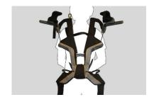
Check to ensure the vertical orientation of the exoskeleton on your back.
