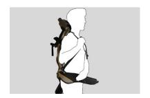
Put on the right shoulder strap like a backpack. While continuing to hold the belt with the left hand to ensure the exoskeleton does not hit your head.
