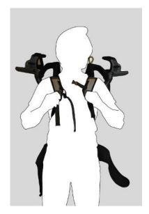
Position the exoskeleton vertically on your back by slightly pulling both shoulder straps up and over your shoulders.
