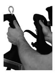
Check play between the two halves of the frame.
