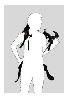
Put on the left shoulder strap, again ensuring that the arms or the rest of the exoskeleton does not hit your head.
