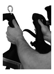
Check Width Adjustment System range and locking. Check the adjustable strap at the back of the SkelEx between the two frame halves.
