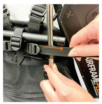
To bring the Spines closer together, pull on both the left and right Straps.
