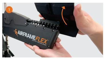
Rotate the Armrest upward to unlock. You will hear a *click*.
