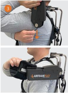
Pull the Lanyard down to release the Latch, then lower the Cassette.
